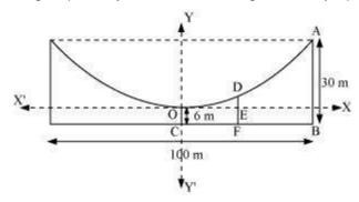
Here, AB and OC are the longest and the shortest wires, respectively, attached to the cable.
